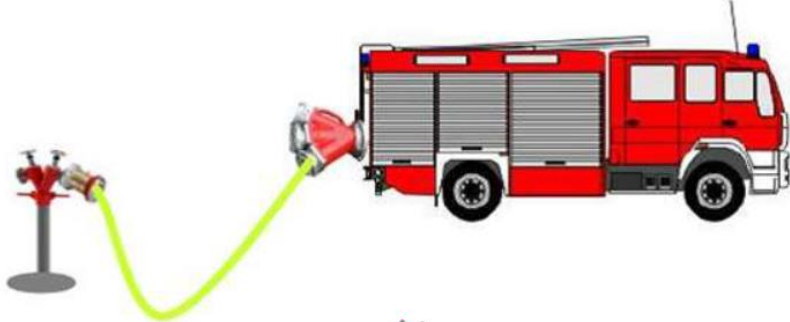
Systemtrenner am Standrohr
